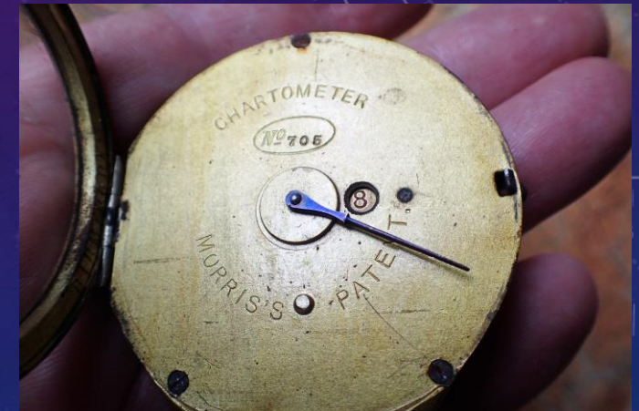
Face of Chartometer without scale card inserted. Revolution counter can be seen to the right of the pointer axis.
