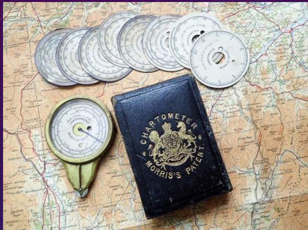
Morris's Patent Chartometer and scale cards with leather bound wooden case
