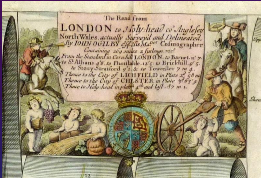
Surveyor and waywiser are shown at the head of Ogilby's 'The Road from London to Holyhead' map. c1698
