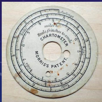
Morris's Patent Chartometer and scale cards with leather bound wooden case
